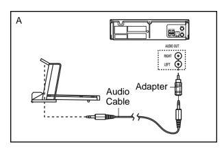
B. Plug one end of the audio cable into the jack beneath the console. Plug the other end of the cable into the included adapter. Plug the adapter into an RCA Y-adapter (available at electronics stores). Next, remove the wire that is currently plugged into the AUDIO OUT jack on your VCR and plug the wire into the unused side of the Y-adapter. Plug the Y-adapter into the AUDIO OUT jack on your VCR.
